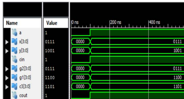
Figure 11: Output waveform of the 4-bit Adder/ Sub-tractor Circuit
